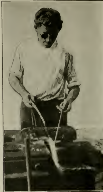
WELDING OPERATOR AT WORK, TORCH IN RIGHT HAND, WELDING ROD IN LEFT.
